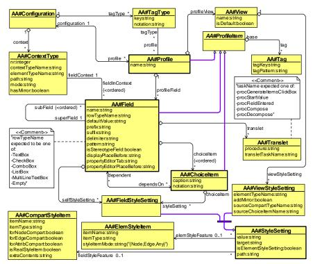
Fig. 3. Visualization profile meta-model
